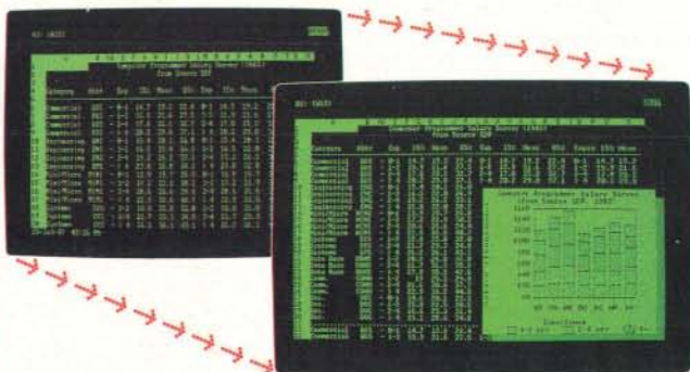
Hercules RamFont lets spreadsheets like 1-2-3 display nearly twice the data with no loss in scrolling speed.
